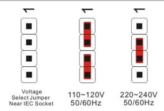
The DAC is designed to be fully regulated in circuit. So, select 110-120V case can also works well in Japan's 100V.
